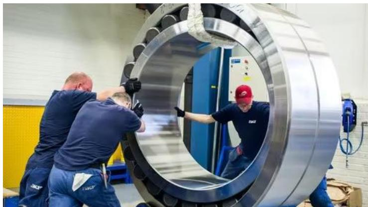
SKF. 8 tonne bearing, diameter of 1.25 m
