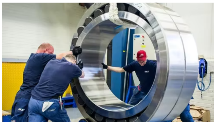
SKF. 8 tonne bearing, diameter of 1.25 m
